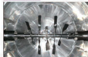
Inner Blade with Oil Spraying Device
